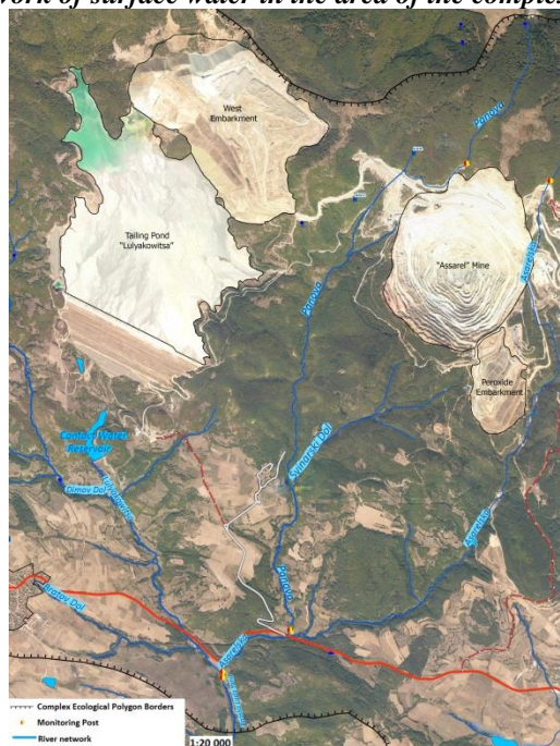
Figure 1. Monitoring network of surface water in the area of the complex ecological polygon (CEP)
