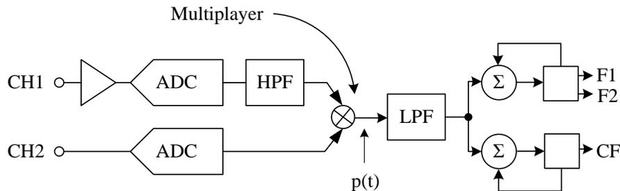
Fig. 2. Functional block diagram of the integral energy meter<sup>2</sup>
