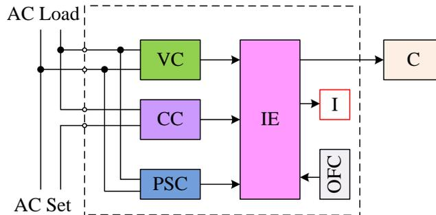
Fig. 1. Block diagram of the electricity metering module
