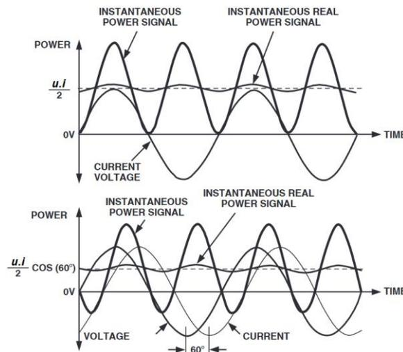
Fig. 3. Diagrams reflecting the determination of the instantaneous power at a power factor  $PF < 1$
