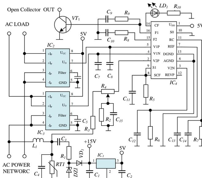
Fig. 4. The electrical circuit diagram of a module for electrical energy measurement
