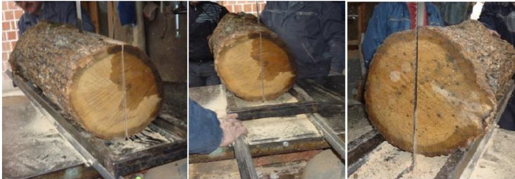
Figure 1. Sawing of the oak logs with band sawing machine.
