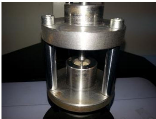
Fig.2. Ceramic specimen testing with fracture strength test
