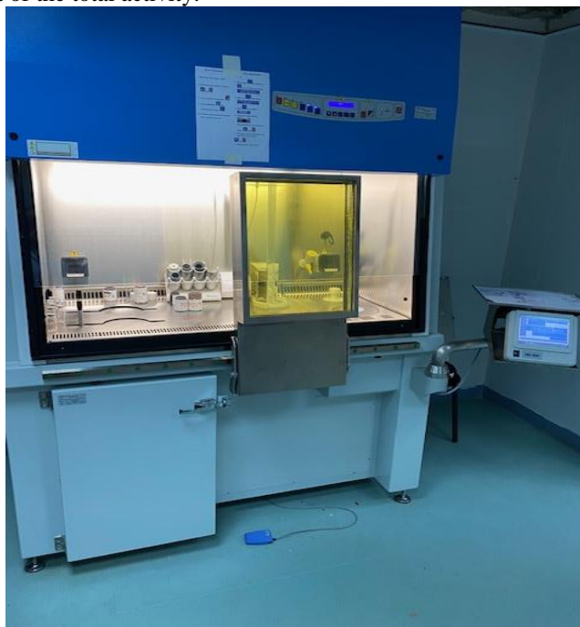
Figure 1. Fume Hood - Safeflow- Class II Biohazard Safety Cabinet in which the procedure of labelling was performed
