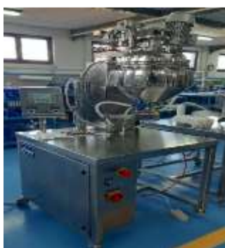
Figure 3. Homogenization mixer of producer OmniProjekt installed in our production site
