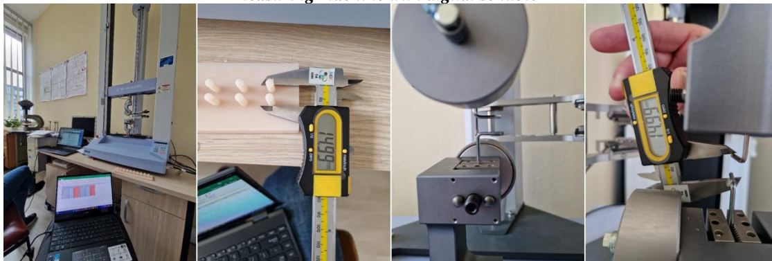
Picture 3. Shimadzu Autograph AGS-X with integrated program for measuring Trapezium X / Measuring of the distal parts of the custom board pins with digital schubler / Measuring the distal parts of the pins in the measuring machine with digital schubler
