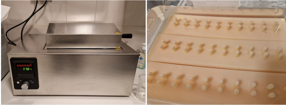
Picture 2. Memmert waterbath WNB 7-45 at 37°C / Elastics put on the custom board with artificial saliva
